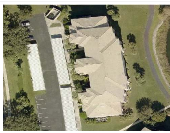
ROOF GEOMETRY – Aerial view of the hip roof shape
